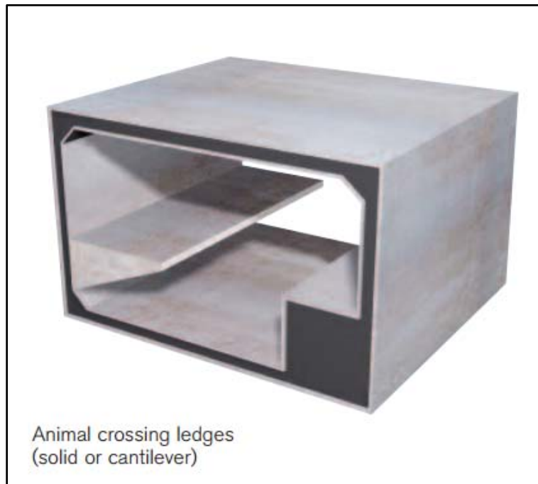
Plate 5: Typical box section with animal crossing ledge (Image courtesy of Hanson Precast)
